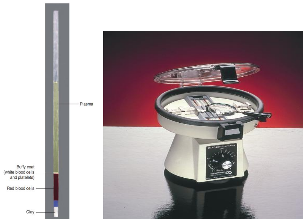
Figure 1.7: Readcrit centrifuge with built-in capillary tube compartments and hematocrit scales. (Courtesy and © Becton, Dickinson and Company, Franklin Lakes, NJ.)
